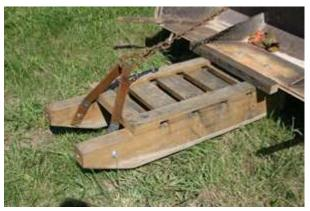
any local nurseries or sod farms cut sod blocks the four inch minimum thickness we wanted. Gregg Caldwell from our building maintenance staff researched and built a sod cutter to use with a tractor. It worked perfectly. After mowing the grass to about four inches in height, our staff was able to cut sod strips twelve inches wide and four inches deep that could then be cut with a spade to the required lengths. Instead of transporting the blocks by team and
