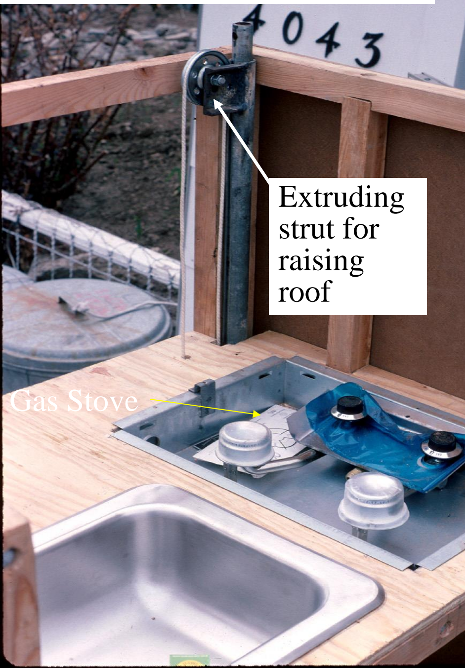
Sink, stove and roof elevator
