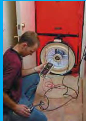
TECHNICIAN PERFORMING A BLOWER DOOR TEST
