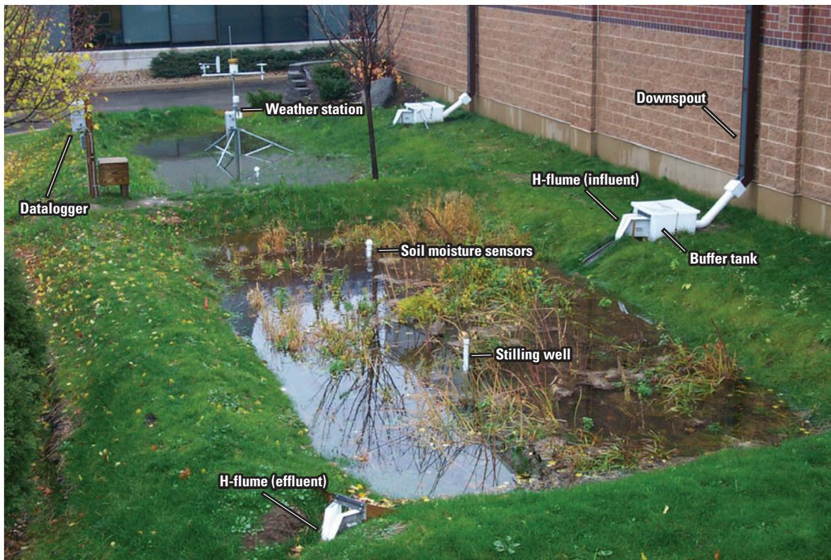
Figure 3. Instrumentation used at the clay rain gardens.
